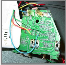
The "clapper LED high rail" is where the **red** wire is attached in this image; this is a common power line that feeds that 3 LED's. The **green** wire is attached to the "2-clap LED ground side", which is the signal from the IC that controls the 2-clap LED. We snipped out all 3 LED's to save current.
