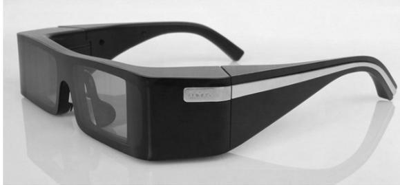
Fig. 3.3 Progress in optical technologies allow displays, such as this prototype from Lumus Ltd., that present information on transparent glass that does not obstruct the wearer's view. Courtesy Lumus Ltd.
