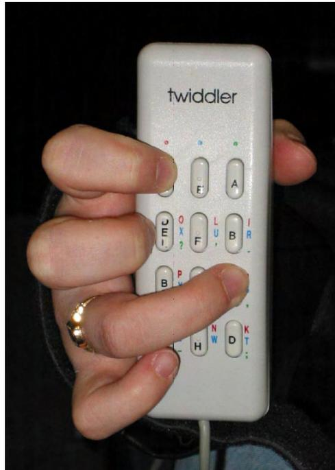
Fig. 2.5 The Twiddler hand-held keyboard allows one-handed, mobile text entry using physical buttons. Image from Lyons et al. [78], © IEEE 2004.
