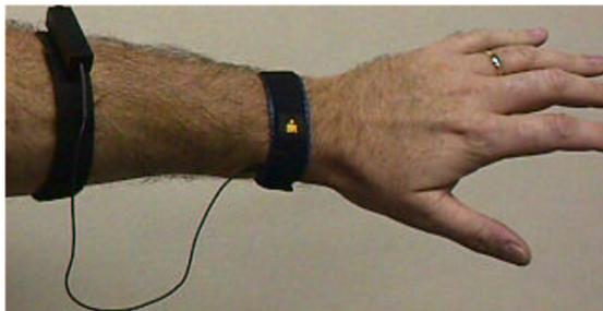
Fig. 2.24 Amento et al. use wrist-mounted microphones to classify gestures based on the unique sounds of various finger gestures [3]. Courtesy Brian Amento.
