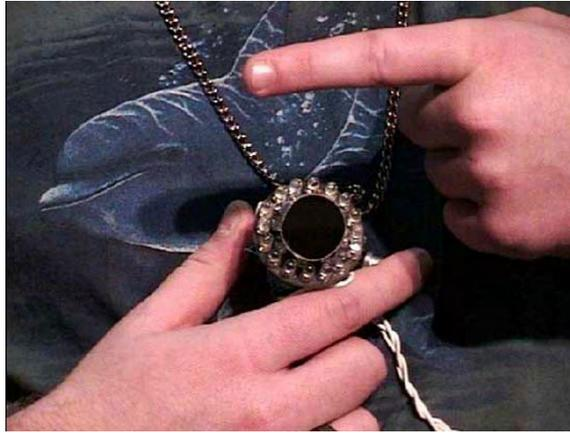
Fig. 2.10 Starner et al.'s Gesture Pendant uses a neck-worn IR camera and emitter for illuminating and sensing the hand [133]. © IEEE 2000.
