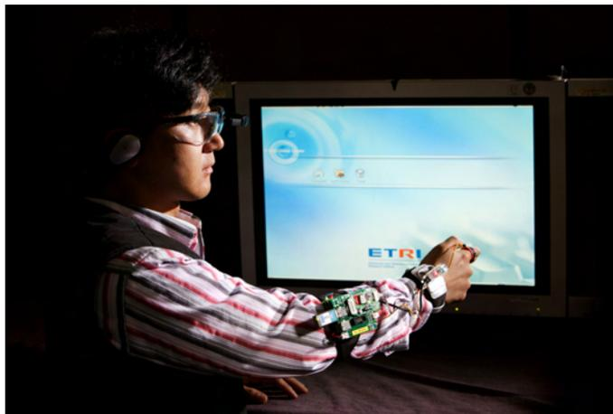
Fig. 2.2 Cho et al. [20] apply lower-power, plane-crossing-based techniques to wrist- and arm-mounted accelerometers. Image courtesy of authors.
