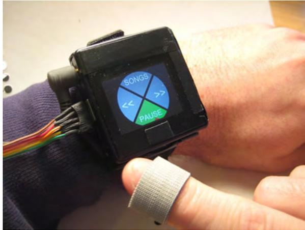
Fig. 2.25 Harrison and Hudson's *Abracadabra* system couples a wrist-mounted magnetometer with a passive magnet worn on the finger to provide three-dimensional input [44]. © ACM 2009.
