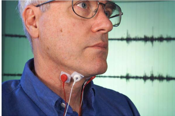
Fig. 2.12 sEMG applied to the throat can recognize the patterns of muscle activation required to control speech production. Image courtesy NASA Ames Research Center, Dominic Hart.
