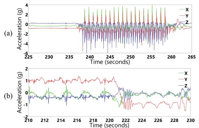
**Figure 1: Challenges separating exercise from non-exercise. (a) The (rare) easy case: a participant goes from a relatively motionless state to rapid movement. (b) A typical case: a participant finishes a set, puts weights down, and stretches a bit; exercise and non-exercise amplitude are almost identical.**
