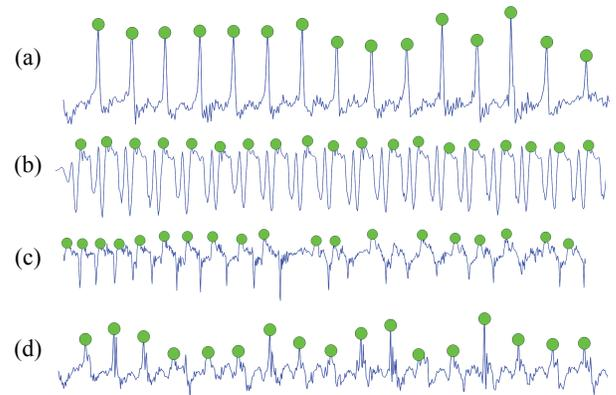
**Figure 2: Counting challenges. (a) Consistent large peaks. (b) Each repetition contains multiple similar peaks. (c) Irregular timing and form. (d) Irregular amplitude. Circles indicate repetitions, correctly identified by our algorithm.**
