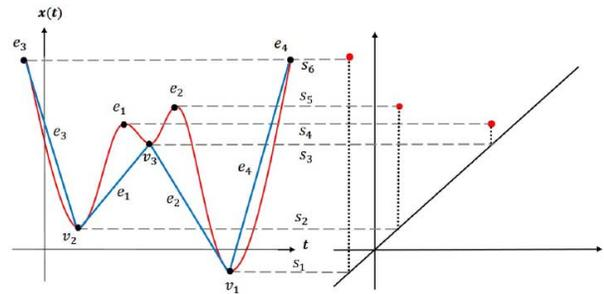
Fig. 2. Construction of a persistence diagram for a single-variable function.
