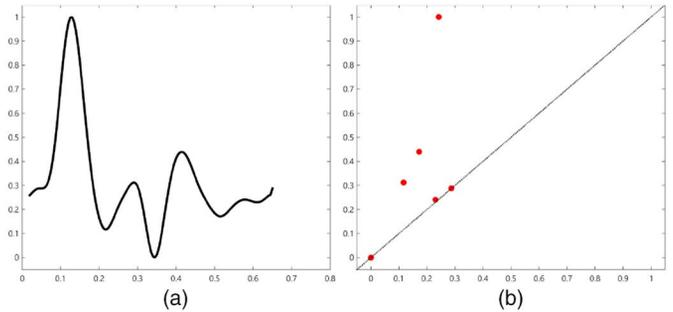
Fig. 3. The first derivative of the pulse pressure wave in Fig. 1 (left) and its persistence diagram (right).
