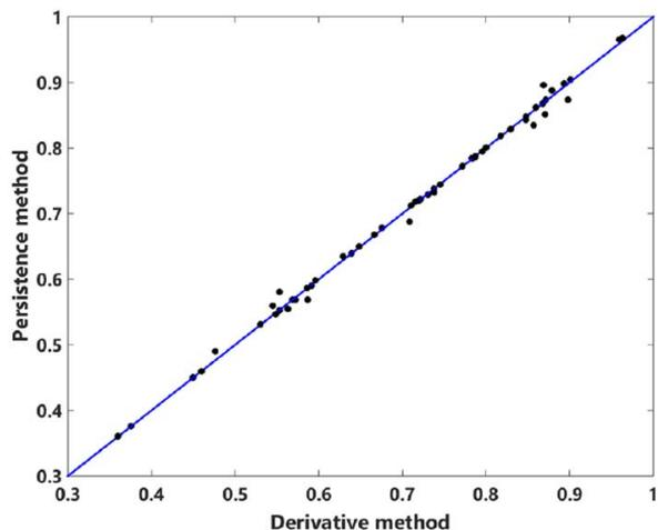
Fig. 5. The correlation between AIx values calculated using the persistence and derivative methods for each of two recordings for all participants. The solid line is  $y = x$ .
