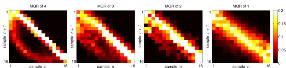
**Figure 3.** Example transition probability distribution functions for various MQRs. Warm colors represent higher probabilities. Color scaling stops at a maximum probability of  $p = 0.20$  to enhance off-diagonal components.
