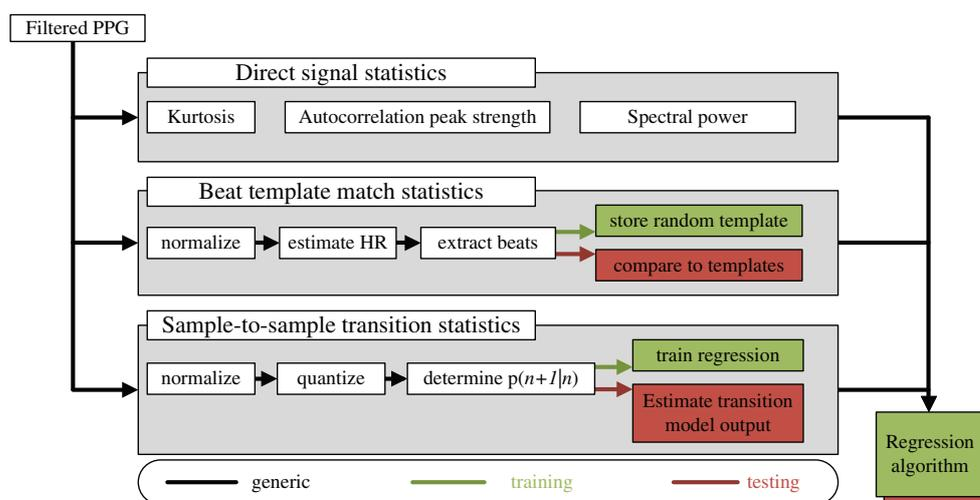
**Figure 2.** Overview of system architecture. After pre-processing, a number of signal statistics or features are derived from each data window of PPG. The majority of these features are used directly by the final regression model, with the exception of the sample-to-sample transition statistics, which first become consolidated in to a single feature using a support-vector regression model.
