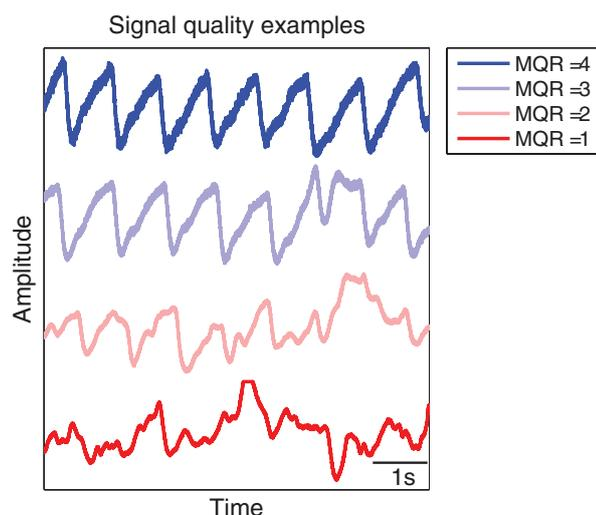
**Figure 1.** Examples of the four classes of manually-rated signal quality. Note the pulse waveform is entirely preserved when MQR = 4 and is preserved to lessening degrees as signal quality decreases.
